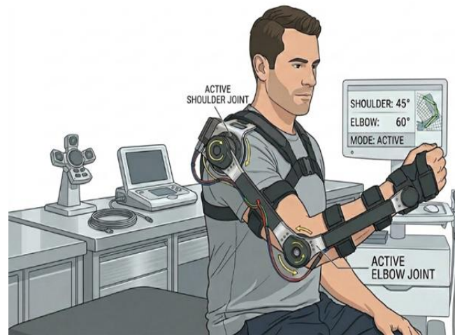
Figure 1 - Experimental setup of the active upper-limb exoskeleton, detailing the integrated active shoulder and elbow joint mechanisms, joint angle readouts, and real-time motion tracking interface described in a virtual world
