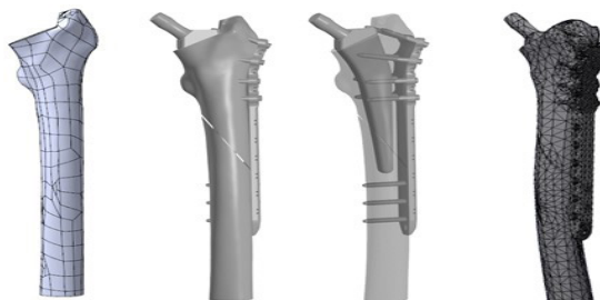
Figure 2 - Computer model and finite element grid of the investigated system "femur – endoprosthesis – periprosthetic plate"
