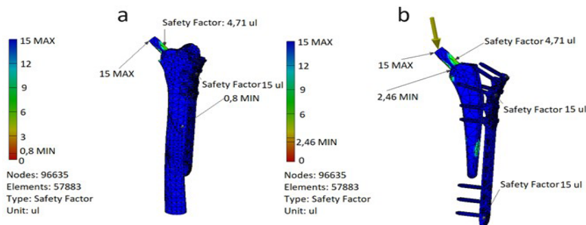
Figure 4 -The stress distribution pattern according to Mises in MPa for: a) the entire femur-endoprosthesis-plate system b) endoprosthesis and plate
