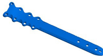
Figure 1 - Plate design for fixation of periprosthetic fractures of the proximal femur
